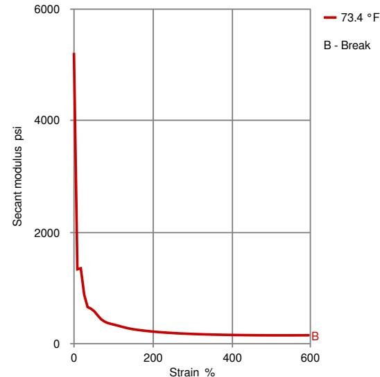
Tested according to ISO 37-1, 500 mm/min
